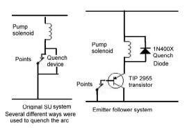
These diagrams show the original SU system and the mods for the emitter follower. Note that when the coil is turned off it generates a large reverse voltage, like an ignition coil. SU quenched this voltage across the points, whilst the quench diode shorts out the reverse voltage in the coil.
