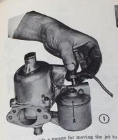
attached to provide a means for moving the jet to correspond to throttle opening and, in some cases, correspond it is attached to a disphragm to provide the main jet is attached to a disphragm to provide the main jet is stached to a disphragm to provide the main jet is attached to a disphragm to provide the main jet is the main terms of the cover, and remove the piston and spring assembly (C).
