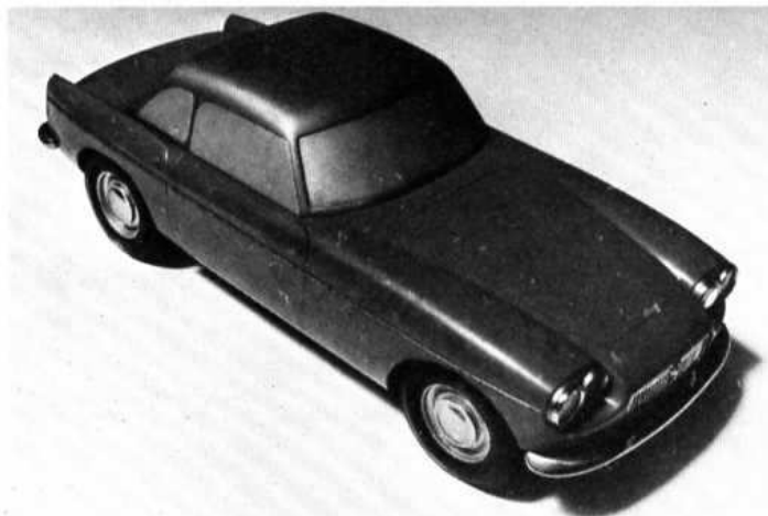
Two wind-tunnel ¼-scale models, above: top, EX186, a streamlined MGA for 1956 with twin-cam and de Dion was built, but not raced; lower, teardrop alternative with supine driver in front behind a large screen. Left, first development of the Frua shape for the MGB – looks almost right apart from twinned headlights
