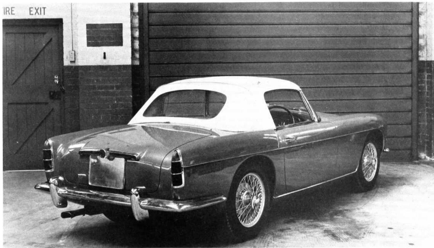
Above and below, the restyled MGA was designed by Abingdon and built by Frua, EX214; some Maserati is evident in grille and boot shape.
