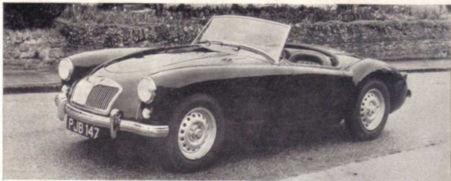
LINES of the twin-cam M.G.A are unchanged, but a distinctive feature is the fitting of centre-lock perforated disc wheels as standard.
