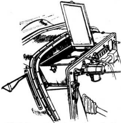
The tool case is in the scuttle under the bonnet. Note the position of the traffic signal.
