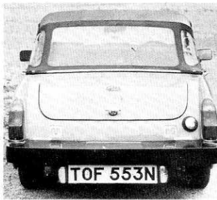
Standard number plate is mounted beneath the new "5 mph" bumper, rather than below the boot lid as in previous Midgets. Reversing lights are standard and boot lid can be left unlocked if the driver wishes
