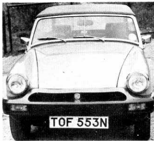
Massive front bumper makes the whole car look bigger than before; inset lights are well protected by lipped extensions. Door mirrors are part of standard equipment. Headlamps are sealed-beam units, not halogen
