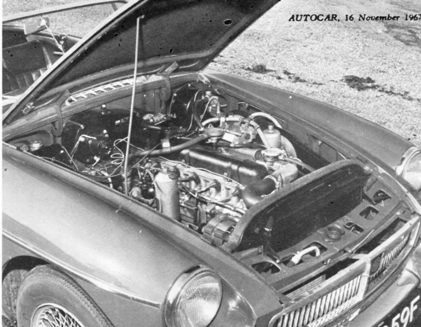
The 6-cyl. engine fills all the available space, but everything needing routine attention is easily reached, especially the oil filter, on the left of the block
