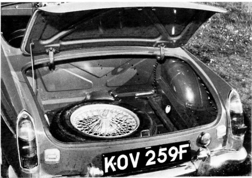
The boot holds a remarkable amount of soft luggage, but there is no trimming. With the hood down the cover and irons take up a good deal of room. A strut has to be used to hold the lid open
