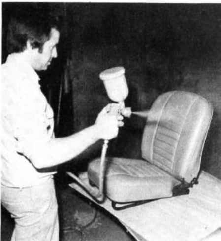
Left, restoring the colour of a leather seat at Charlton Street. Above, the hide being automatically stretched. Below, left, familiar names; the bins contain the upholstery dyes. Below, the machine that measures the square footage of the hides.
