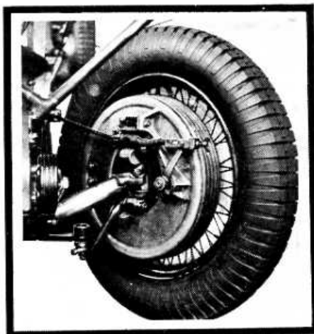
On the M.G. Mark III the axle ends and steering arms are polished to facilitate inspection for flaws.
